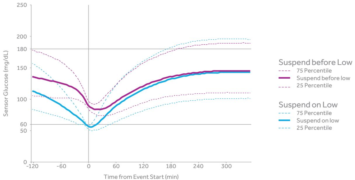
FIG. 2. SG trajectories associated with enabled event start time (min) for "suspend before low" and "suspend on low" features. The graph shows median SG values for suspension events of any duration for which the low limit was set to 60 mg/dL.
